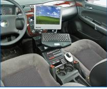
**Stout Mount™ Console**Versatile design allows for endless equipment configurations. Innovative swing-arm keyboard mounting. *C-SM-830*
